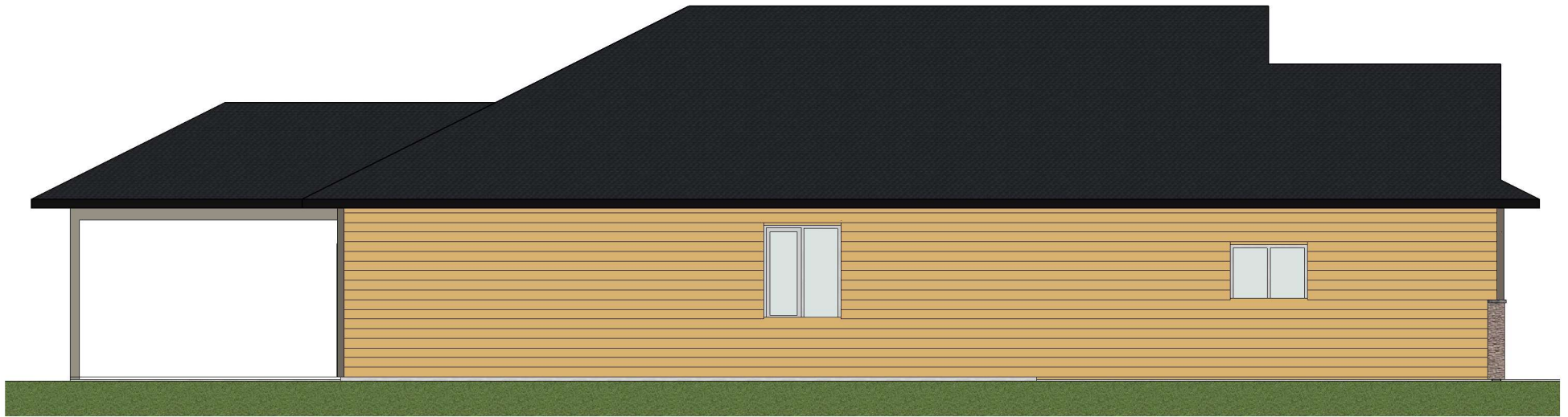
④ West Elevation 1/8" = 1'-0"
